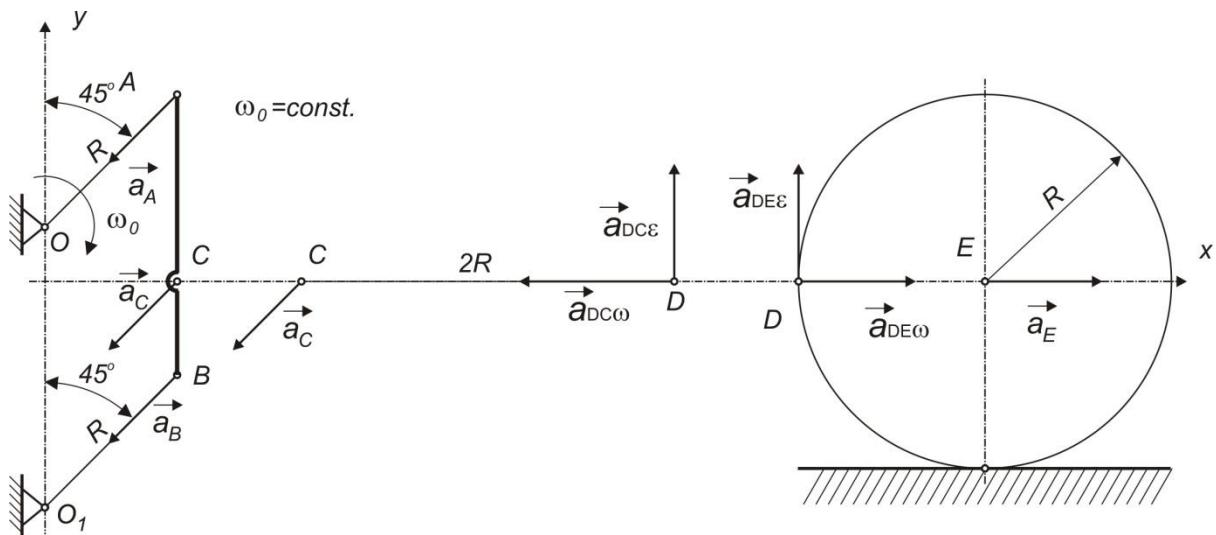
$$\vec{a}_C = -\frac{\sqrt{2}}{2} a_{C\omega} \vec{i} - \frac{\sqrt{2}}{2} a_{C\omega} \vec{j} = -\frac{\sqrt{2}}{2} R \omega_0^2 \vec{i} - \frac{\sqrt{2}}{2} R \omega_0^2 \vec{j}$$
